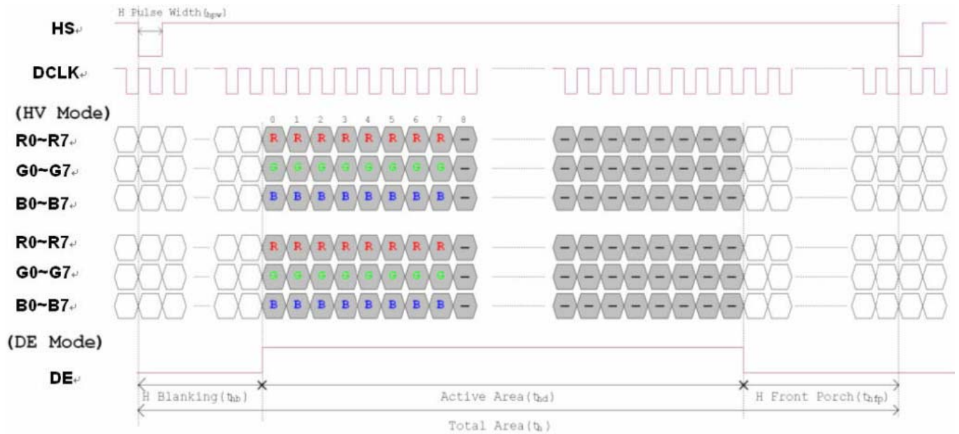
Figure 3.1 Horizontal input timing diagram
